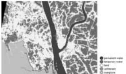
Fig. 6. Result of data and sensor fusion from RADARSAT and ASTER data
